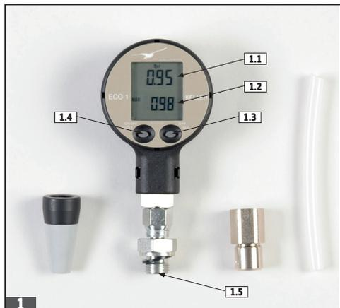
The digital manometer has two control buttons:
