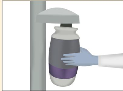
2. Connect bottle to the dental unit and flood the water pipes with GREEN&CLEAN BR.
