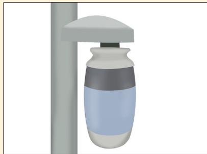
5. Fill the bottle with clean water, reconnect to the unit and rinse the water lines completely.
