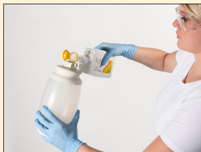
5. Pour GREEN&CLEAN WK into the water bottle and reconnect it to the dental unit
